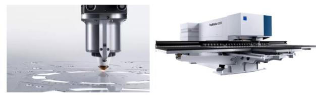
Our TruMatic combines the punching and laser processing of your components and offers a wide range of processing for components with complex geometries. Standard contours, deformations and threads are produced with the punching head and filigree outer and inner contours with the laser.
