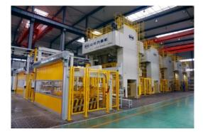
For the production of prototypes and small series, we have deep drawing presses from 100 to 300 tons. We ensure the production of large series in one of our pressing plants in China. Here we have transfer presses and presses with decoiling systems from 100 to 1,280 tons.
